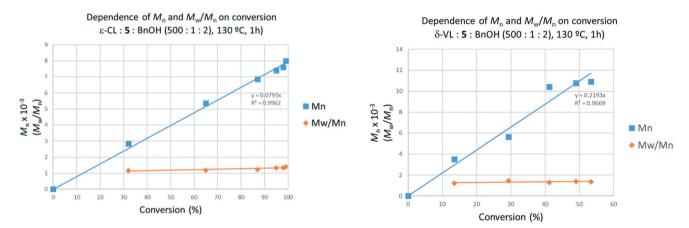
Fig. 12 Dependence of  $M_n$  and polydispersity on conversion in the ROP of cyclic esters catalyzed by 5. Left:  $\varepsilon$ -CL; right:  $\delta$ -VL.
