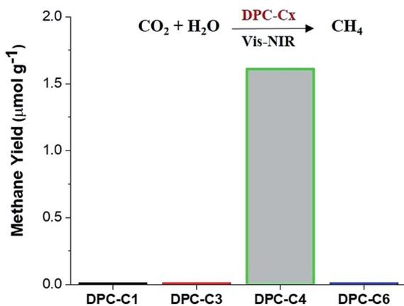
Fig. 11 Photocatalytic CO<sub>2</sub> conversion to methane using DPC-C1, DPC-C3, DPC-C4, and DPC-C6 as catalysts under light (400 to 1100 nm). No conversion in the dark or in the absence of CO<sub>2</sub>. Micro-GC with TCD sensitivity >10 ppm. Error in methane yield for DPC-C4: ±0.51.
