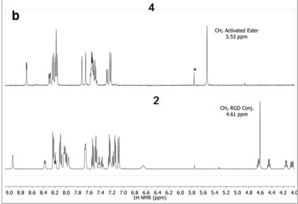
Scheme 1 Synthesis of bio-responsive cRGD NIR-AZA conjugate 2. (a) Conditions for activated ester/amine coupling of 4 and 5. (b)  $^{1}$ H NMR spectra of 4 and 2 with key methylene peaks (shown in blue) indicated (\*CH<sub>2</sub>Cl<sub>2</sub>).
