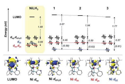
Fig. 6 (Top) MO diagrams of NiLH<sub>3</sub> and complexes 1–3. The ligand field energies (in eV) are based on UV-Vis data (Table 5). TD-DFT calculated energies are shown (in eV, italicized within parentheses) when experimental values were not obtainable. (Bottom) MOs for complex 2, which are representative of those for the series. Note that MO energies are drawn to scale, but energy comparisons across the complexes are qualitative.
