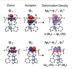
Fig. 4 The two dominant NOCV pairs in 3-H<sub>2</sub> and their associated deformation densities ( $\Delta\rho_1$ , top right;  $\Delta\rho_2$ , bottom right; contour isovalue = 0.04 a.u.). The colors of the deformation densities indicate the flow of electrons, from red to blue, involved in the Ni-H<sub>2</sub> interaction.
