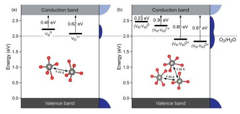
Fig. 3 Defect ionisation levels of oxygen vacancies in different charge states calculated from hybrid density functional theory for (a) an isolated oxygen vacancy  $V_O(y)$  and (b) a defect complex composed of two oxygen vacancies  $V_O(zy)$ . Energies are relative to the valence band edge. Densities of states are illustrated schematically at the right side of each panel. The insets show local atomic structures and the distance between the W atoms
