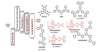
Scheme 2 Energy level diagram of the HOMO and LUMO levels of materials investigated and their chemical molecular structures.
