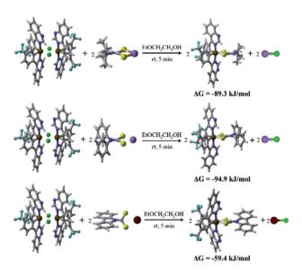
Fig. 1 The calculated Gibbs free energy change  $\Delta G$  of the three reactions of (4tfmpq)<sub>2</sub>Ir(dipdtc), (4tfmpq)<sub>2</sub>Ir(dpdtc) and (4tfmpq)<sub>2</sub>-Ir(Czdtc) complexes.
