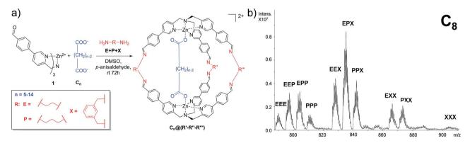
Fig. 2 (a) DCL using different linkers E, P and X. The ratio between the complex, guest, linkers and p-anisaldehyde is 2:1:9:12 ([1] = 1.6 mM,  $[C_n] = 0.8$  mM, and [E] = [P] = [X] = 2.4 mM [p-anisaldehyde] = 9.5 mM). (b) ESI-MS spectrum of the mixture in the presence of  $C_8$  as the guest after 72 hours.
