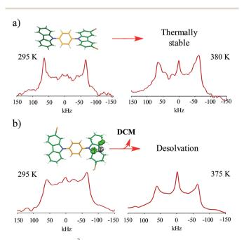
Fig. 4 Experimental <sup>2</sup>H NMR line shapes of (a) compound 1 and (b) compound 4 at the indicated temperatures.
