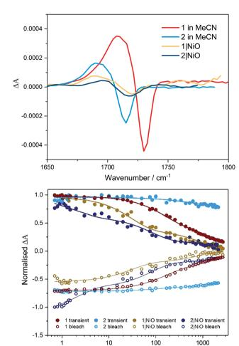
Fig. 4 TRIR Spectra (top, 1 ps) and kinetic traces (bottom) for 1 (red) and 2 (light blue) in CD<sub>3</sub>CN and 1|NiO (yellow) and 2|NiO (dark blue) following excitation ( $\lambda=470$  nm). On the bottom figure, the symbols represent data points (open = bleach, filled = transient absorption) and the lines are the exponential fit to the data.
