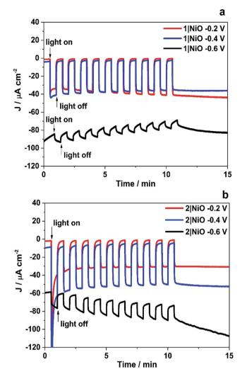
Fig. 7 Chronoamperometry measurements of 1|NiO (a) and 2|NiO (b) immersed in pH 3 buffer containing 0.1 M potassium hydrogen phthalate.  $E_{appl} = -0.2 \text{ V}$ , -0.4 V and -0.6 V vs. Ag/AgCl (3.0 M NaCl). Chopped light illumination was applied with 30 s intervals (10 cycles of dark current/photocurrent)
