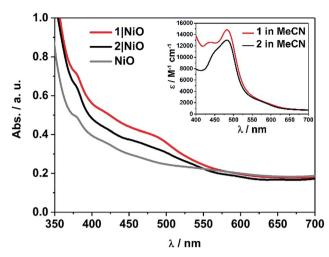
Fig. 2 UV-vis absorption spectra of  $\bf 1$  (red) and  $\bf 2$  (black) adsorbed on NiO and bare NiO (gray). Inset: UV-vis absorption spectra of  $\bf 1$  (red) and  $\bf 2$  (black) in MeCN (0.028 mM and 0.032 mM, respectively).
