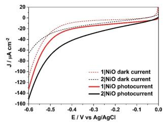
Fig. 6 Linear sweep voltammograms of 1|NiO and 2|NiO immersed in aqueous 0.1 M KCl electrolyte (pH 3). The potential was sweet from  $E_{\rm appl} = 0$  to -0.6 V vs. Ag/AgCl (3.0 M NaCl) in the dark and under simulated light illumination (AM1.5, 100 mW cm<sup>-2</sup>).
