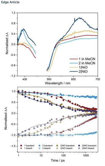
Fig. 3 Transient absorption spectra (top, 1 ps) and kinetic traces (bottom) for 1 (red) and 2 (light blue) in CD<sub>3</sub>CN and 1|NiO (yellow) and 2|NiO (dark blue) following excitation ( $\lambda=470$  nm) probed at 490 nm (bleach, open symbols) and 620 nm (transient, filled symbols). On the bottom figure, the rings represent data points and the lines are the exponential fit to the data.
