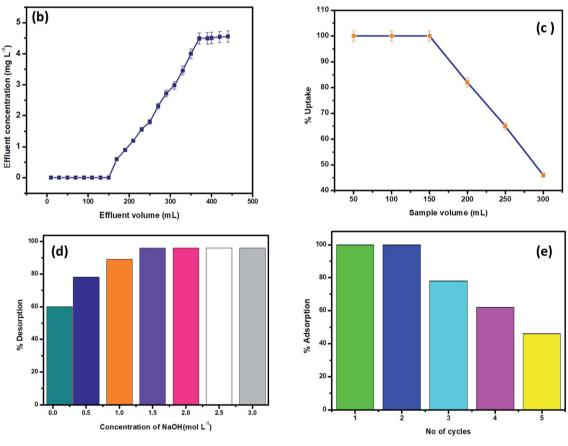
Fig. 7 (a) Diagrammatic representation of column setup for Cr(v<sub>1</sub>) treatment (b) breakthrough curve (c) effect of sample volume (d) effect of varied NaOH concentrations (e) regeneration efficiency of the biosorbent.
