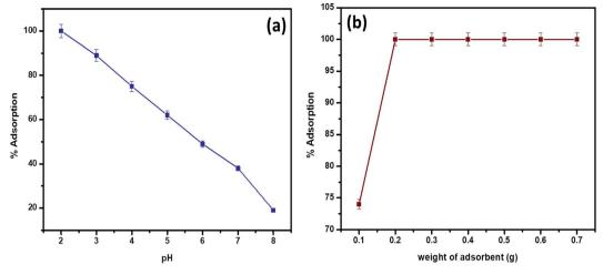
Fig. 5 (a) pH effect on biosorption (at 30 °C, 5 mg  $L^{-1}$  Cr(v<sub>i</sub>)) (b) variation of adsorbent dosage (at pH 2.0, 30 °C, 5 mg  $L^{-1}$  Cr(v<sub>i</sub>)).
