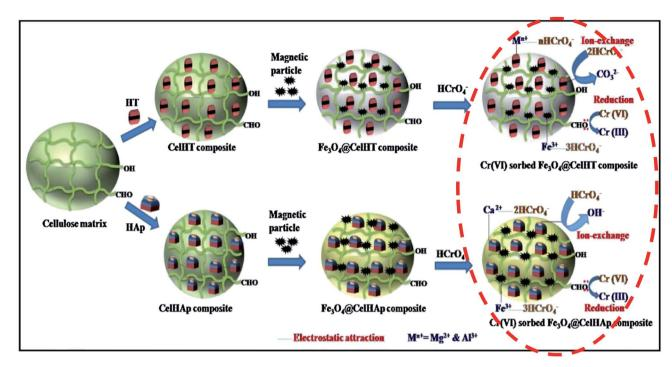
Fig. 3 A possible Cr(vi) sorption mechanism pathway onto magnetic particles imprinted cellulose-based biocomposites. Chromium removal and reduction are occurring at the last step indicated in red, while the other steps show the preparation of biocomposites. Copied from ref. 36, with permission from Elsevier and modified.
