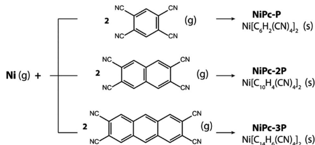
Scheme 1 Co-evaporation of Ni and the corresponding tetracyano linkers resulting in single-layer NiPc-P, NiPc-2P, and NiPc-3P.
