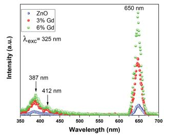
Photoluminescence spectra of pure ZnO and ZnO: Gd (3% and Fig. 7 6%).
