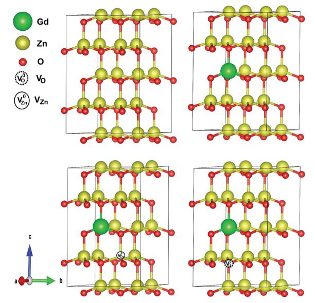
Fig. 9 Crystal structures of pristine, Gd-doped ZnO and Gd-complex defects ZnO
