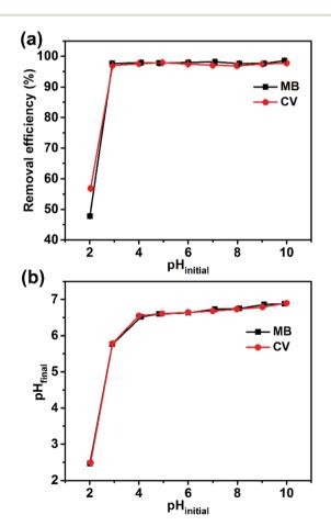
Fig. 5 (a) Effect of initial solution pH on the removal efficiency by the Dex-MA/PAA hydrogel and (b) finial pH changes after adding the Dex-MA/PAA hydrogel. Dex-MA/PAA hydrogel dose: 1 g L $^{-1}$ , dye concentration: 50 mg L $^{-1}$ , contact time: 3 h.
