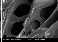
Fig. 4 SEM images of the fracture surface of the freeze-dried Dex-MA/PAA hydrogel at two magnifications.
