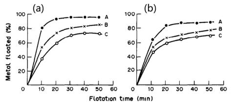
Fig. 8 Effects of flotation time and surfactants on  $R_{Rh}$  (a),  $R_{Pd}$  (b) recovery: A SDBS, B SDS, C sodium lauryl sulfate (SLS). Reproduced from ref. 13 with permission from Elsevier, Copyright 1991. Reprinted from X. He, Ion flotation of rhodium(III) and palladium(III) with anionic surfactants, *Talanta*, 38, 319–323, Copyright (1991), with permission from Elsevier.
