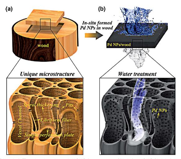
Fig. 9 (a) Schematic of a 3D wood membrane decorated with Pd NPs for water treatment. (b) *In situ* formed Pd NPs (black dots) within the wood demonstrated he plasmonic effect inside the wood channels. <sup>107</sup> This figure has been adapted from ref. 107 with permission from ACS Nano.
