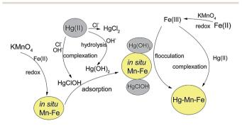
Fig. 4 Schematic diagram of the mechanisms of Hg(II) removal by in situ Mn-Fe.55 This figure has been adapted from ref. 55 with permission from Elsevier.
