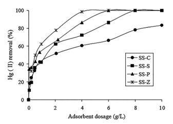
Fig. 2 Effect of adsorbent dosage on Hg(II) removal.  $(Hg^{2+} 200 \text{ mg L}^{-1}, \text{ pH } 5.0, \text{ time } 7 \text{ h, } 25 ^{\circ}\text{C.}) \text{ SS-S, SS-P, SS-Z and SS-C represented activated carbons treated by <math>H_2SO_4$ ,  $H_3PO_4$ ,  $ZICl_2$  and that with no treatment. <sup>28</sup> This figure has been adapted from ref. 28 with permission from Elsevier.
