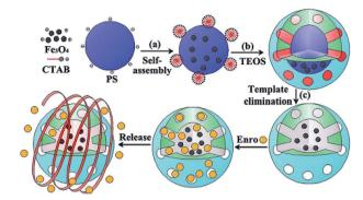
Schematic of the ENR loading and release of MHMS.71
