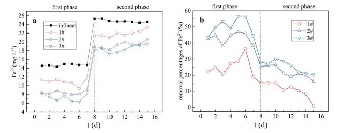
Fig. 6 (a)  $Fe^{2+}$  residual concentration in Columns 1, 2, 3. (b) The removal percentage of  $Fe^{2+}$  in Columns 1, 2, 3. Influent is the  $Fe^{2+}$  concentration in influent water of AMD. 1#, 2# and 3# in (a) are the residual Fe<sup>2+</sup> concentration in AMD after repairing AMD with Column 1, Column 2 and Column 3 respectively. 1#, 2# and 3# in (b) are the removal percentage of Fe<sup>2+</sup> in AMD by the three dynamic columns corresponding to (a) respectively.
