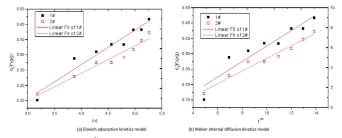
Fig. 11 Kinetic curves of adsorption Fe<sup>2+</sup> by immobilized particles. 1# is modified corncob fixed SRB sludge particles, 2# is unmodified corn cob fixed SRB sludge particles.
