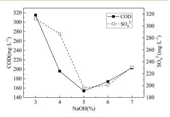
Fig. 3 COD release and  ${\rm SO_4}^{2-}$  residual concentration under different NaOH concentration. The  ${\rm H_2O_2}$  concentration was 1.5%.the modification time was 24 h.
