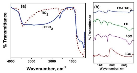
Fig. 3 FT-IR spectra of (a) air- and H<sub>2</sub>-annealed TiO<sub>2</sub>, and (b) pristine graphite, SGO, FG, HTIO<sub>2</sub> and FG-HTiO<sub>2</sub>.
