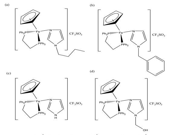
Fig. 50 Chemical structure of the (a)  $[Fe(\eta^5-cp)(dppe)(1-Bulm)]CF_3SO_3$ , (b)  $[Fe(\eta^5-cp)(dppe)(1-Bl)]CF_3SO_3$ , (c)  $[Fe(\eta^5-cp)(dppe)(1-Hmlm)]CF_3SO_3$  and (d)  $[Fe(\eta^5-cp)(dppe)(1-Hmlm)]CF_3SO_3$  complexes.
