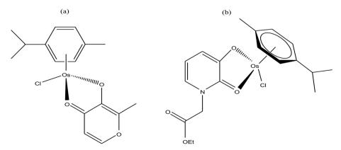
Fig. 56 Chemical structure of the osmium-arene complexes (a)  $[M(\eta^6-p\text{-cym})(\text{mal})\text{Cl}]$  and (b)  $[Os(\eta^6-p\text{-cymene})(\text{NEHP})\text{Cl}]$  containing an anionic O,O-chelating ligand.
