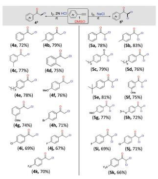
Scheme 3 Scope of mono- and di-oxychlorination. Reaction conditions:  $^{a}$ arylacetylene **1** (1.0 mmol), I<sub>2</sub> (2.2 mmol), and 2 N HCl (0.5 mL) in 3 mL of DMSO at r.t. for 16 h. <sup>b</sup>Arylacetylene **1** (1.0 mmol), I<sub>2</sub> (2.2 mmol), and NaCl (2.0 mmol) in 3 mL of DMSO at r.t. for 4 h.
