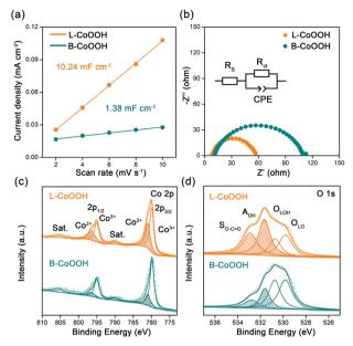
Fig. 3 Origin of the excellent OER activity of L-CoOOH. (a) The relationship between the current density and the scan rate. (b) The EIS of L-CoOOH and B-CoOOH recorded at a potential of 1.56  $V_{\rm RHE}$ . (c) Co 2p and (d) O 1s XPS spectra of L-CoOOH and B-CoOOH.
