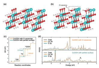
Fig. 4 DFT calculations of CoOOH with a perfect surface and CoOOH with oxygen vacancies. The structure models of (a) a perfect CoOOH (012) surface and (b) a CoOOH (012) surface with oxygen vacancies. Color code: white for H, red for O, and cyan for Co. (c) The free energy profile for the OER pathway and (d) PDOS of the perfect surface and the surface with oxygen vacancies.
