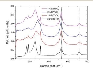
Fig. 9 Composition-dependent Raman spectra of BiYbO<sub>3</sub> and LaYbO<sub>3</sub>-doped barium titanate at −180 °C.
