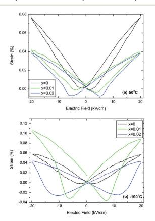
Fig. 4 Electric-field induced strain at (a) 50 °C and (b) -100 °C for (1 - x)BaTiO $_3$ -xBiYbO $_3$  ceramics.
