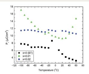
Fig. 3 Temperature dependence of the remanent polarisation,  $P_r$ , for  $(1 - x)BaTiO_3 - xBiYbO_3$  ceramics.
