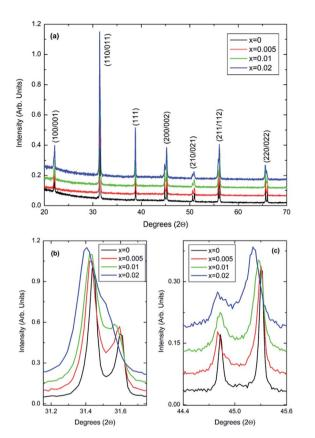
Fig. 1 (a-c) Room-temperature XRD data for  $(1 - x)BaTiO_3 - xBiYbO_3$ ceramics in the  $0 \le x \le 0.02$  range
