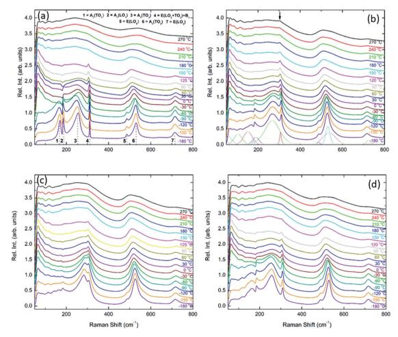
Fig. 7 In situ Raman spectroscopy for (a) undoped BaTiO<sub>3</sub>, (b) 1 mol% doped BiYbO<sub>3</sub>, (c) 2 mol% doped BiYbO<sub>3</sub> and (d) 1 mol% doped LaYbO<sub>3</sub>.
