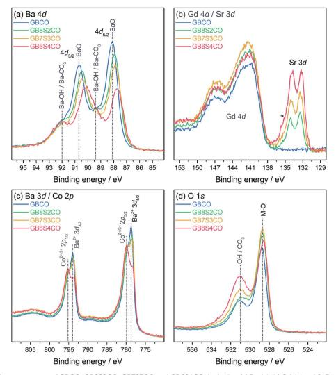
Fig. 5 X-ray photoelectron spectra of GBCO, GB8S2CO, GB7S3CO and GB6S4CO, including (a) Ba 4d, (b) Gd 4d and Sr 3d (\* = Sr-OH/Sr-CO<sub>3</sub>), (c) Ba 3d and Co 2p, and (d) O 1s core level spectra.
