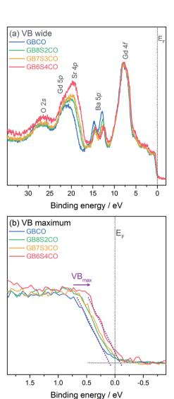
Fig. 6 X-ray photoelectron spectra of GBCO, GB8S2CO, GB7S3CO, and GB6S4CO, including (a) wide valence region, and (b) an expanded view around the valence band maximum VB<sub>max</sub>. Linear fits to the background and  $VB_{max}$  are shown as dotted lines in (b). The dotted line at 0 eV indicates the position of the Fermi energy  $E_{\rm F}$ .
