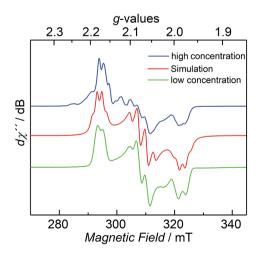
Fig. 3 CW X-band EPR spectrum of 2 at 7 K with different concentrations (blue and green trace), and its simulation (red trace), see ESI† for details.
