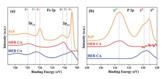
Fig. 8 (a) Fe 2p and (b) P 2p XPS spectra of as-synthesized FeP and after the electrochemical OER and HER treatment. The respective oxidation states of both Co and P are represented in dashed lines (see main text).
