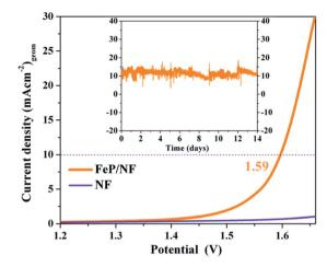
Fig. 9 LSV curves of water electrolysis for FeP||FeP on NF as anode and cathode in a two-electrode cell (sweep rate 1 mV s<sup>-1</sup>) and (inset) the stability tests of corresponding electrolysis at an applied bias of 1.6 V maintaining the current of 10 mA (cm)<sup>-2</sup> over a period of 14 days.
