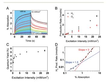
Fig. 6 Photocatalytic and PIAS analysis of GaN:ZnO + cocatalyst samples. (A) PIAS kinetic traces monitored at 610 nm. (B) Production rates of  $\rm H_2$  and  $\rm O_2$  and (C) water splitting quantum yield as a function of 365 nm LED excitation intensity. (D) Rate law analysis of overall water splitting. The  $\rm H_2$  production rate is plotted as a function of the optical signal observed at 610 nm after 45 s of LED irradiation at different excitation intensities, as shown in panel (A).
