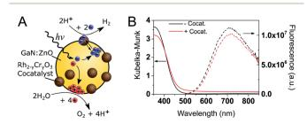
Fig. 1 (A) Schematic of GaN:ZnO/Rh<sub>2-y</sub>Cr<sub>y</sub>O<sub>3</sub> photocatalytic overall water splitting system. (B) Steady-state diffuse reflectance (left, solid lines) and PL (right, dotted lines.  $\lambda_{\rm ex.}=355$  nm) spectra of GaN:ZnO samples under air without (black) and with (red) Rh<sub>2-y</sub>Cr<sub>y</sub>O<sub>3</sub> cocatalyst.
