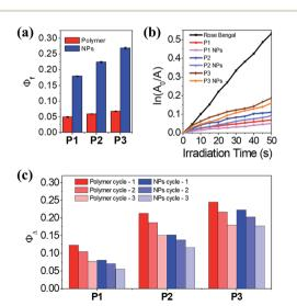
Fig. 4 (a)  $\Phi_{\rm f}$  of P1-P3 and the P1-P3 NPs in HEPES buffer (10 mM, pH 7.0) at 25 °C. (b) Plot of  $ln(A_0/A)$  as a function of time of visible light irradiation on the various photosensitizers, where  $A_0$  and A are absorption intensity at 400 nm at the beginning and at irradiation time t, respectively. (c)  $\Phi_{\Delta}$  of P1-P3 and the P1-P3 NPs in HEPES buffer/  $D_2O(V/V = 1:9)$
