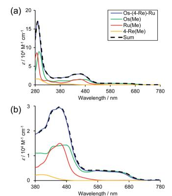
Fig. 3 UV-Vis absorption spectra of the obtained trinuclear complex (a) Os-(4-Re)-Ru (blue) and the corresponding mononuclear complexes, *i.e.* Os(Me) (green), Re(Me) (yellow) and Ru(Me) (red). The 1:1:1 summation spectrum of Os(Me), 4-Re(Me) and Ru(Me) is illustrated as a dotted line. The solvent was MeCN. (b) Enlarged spectra at  $\lambda_{\rm abs}=380$  to 780 nm.
