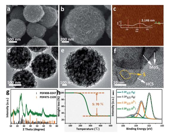
Fig. 2 (a and b) FESEM, (d-f) TEM images, (g) XRD, (h) TGA and (i) XPS spectra of the S/MoS<sub>2</sub>@HCS composite. (c) AFM image of the MoS<sub>2</sub>@HCS composite after a sonication treatment.
