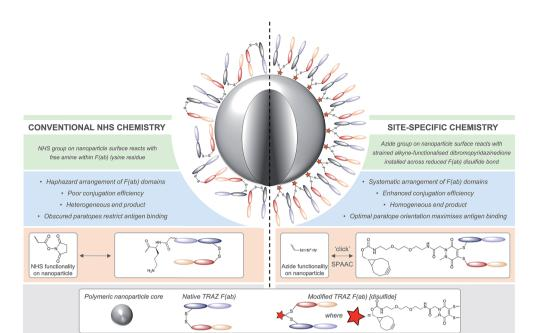
Fig. 1 Comparison of site-specific conjugation approach *versus* conventional NHS coupling. Use of a novel heterobifunctional linker permits the controlled assembly of a surface corona of F(ab) targeting ligands on nanoparticles. The concentrated display of oriented and accessible paratopes afforded by this approach maximises target interactions, leading to significantly enhanced avidity *versus* conventional coupling chemistries
