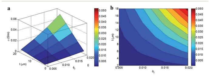
Fig. 3 (a) 3D and (b) contour patterns for the influences of " $\phi_f$ " and "l" parameters on the conductivity of nanocomposites at average levels of other variables.
