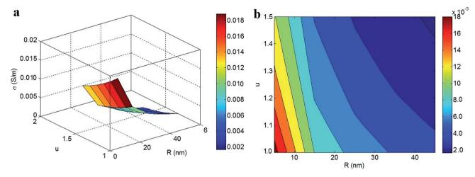
Fig. 4 Roles of "R" and "u" parameters in the conductivity of nanocomposites at average levels of other parameters: (a) 3D and (b) contour plots.
