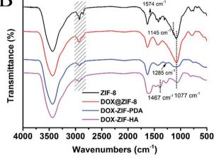
Fig. 4 (A) Surface zeta potential and (B) FTIR spectra of the prepared nanoparticles in different stages.
