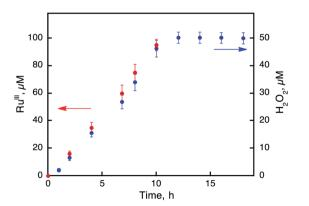
Fig. 3 Time courses of the concentrations of  $[Ru^{III}(Me_2phen)_3]^{3+}$  (red) and  $H_2O_2$  (blue) produced from  $H_2O$  and  $O_2$  in the photocatalytic oxidation of  $[Ru^{II}(Me_2phen)_3]^{2+}$  by  $O_2$  under photoirradiation (white light) of an air-saturated solvent mixture of MeCN and  $H_2O$  (v/v = 23:2) containing  $[Ru^{II}(Me_2phen)_3]^{2+}$  (100  $\mu$ M) in the presence of  $Sc(NO_3)_3$  (100 mM) at 298 K.
