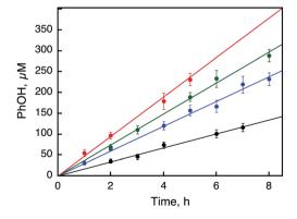
Fig. 6 Time courses of the catalytic hydroxylation of benzene to PhOH with  $H_2O_2$  (1.0 mM) in the presence of 1 [10  $\mu M$  (black), 50  $\mu M$  (blue), 100  $\mu M$  (green), and 500  $\mu M$  (red)] in a solvent mixture of MeCN and  $H_2O$  (v/v =23:2) containing benzene (1.0 M) and Sc(NO<sub>3</sub>)<sub>3</sub> (100 mM) at 298 K.
