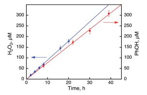
Fig. 7 Time courses of the products from the photoinduced reaction under photoirradiation (white light) in an  $O_2$ -saturated solvent mixture of MeCN and  $H_2O$  (v/v = 23 : 2) containing 1 (0.50 mM), [Ru<sup>II</sup>(Me<sub>2</sub>-phen)<sub>3</sub>]<sup>2+</sup> (0.10 mM), and Sc(NO<sub>3</sub>)<sub>3</sub> (100 mM) in the absence (blue) and presence (red) of benzene (1.0 M) at 298 K.
