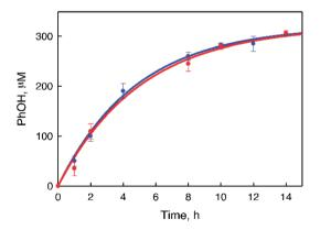
**Fig. 2** Time courses of PhOH concentration produced in the photocatalytic oxidation of benzene under photoirradiation (white light) of an  $O_2$ -saturated solvent mixture of MeCN and  $H_2O$  (v/v = 23:2) containing **1** (0.10 mM),  $[Ru^{II}(Me_2phen)_3]^{2+}$  (1.0 mM), and benzene (1.0 mM, blue circles) or benzene- $d_6$  (1.0 mM, red circles) in the presence of  $Sc(NO_3)_3$  (100 mM) at 298 K. No p-benzoquinone was produced under the present experimental conditions.
