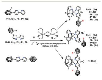
Scheme 2 The synthetic routes of o-carborane modified iridium(III) complexes: (i) CH<sub>2</sub>Cl<sub>2</sub>/CH<sub>3</sub>OH (1:1, v/v), refluxing overnight, KPF<sub>6</sub>.
