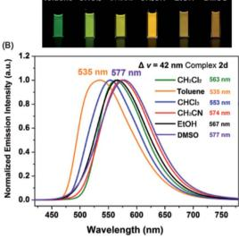
Fig. 3 (A) Luminescence photographs of 2d in various solvents. (B) Phosphorescence spectra of complex 2d in toluene (0.36 D), chloroform (1.04 D), dichloromethane (1.60 D), acetonitrile (3.84 D), ethanol (1.69 D), and DMSO (3.96 D).
