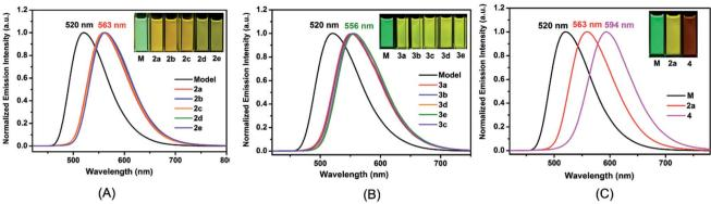
Fig. 2 PL spectra of iridium(III) complexes: (A) complexes 2a, 2b, 2c, 2d, 2e, and Model; (B) complexes 3a, 3b, 3c, 3d, 3e, and Model in degassed  $CH_2Cl_2$  (1.0  $\times$  10<sup>-5</sup> M) at room temperature. (C) PL spectra of iridium(III) complexes Model, 2a, and 4 in degassed  $CH_2Cl_2$  (1.0  $\times$  10<sup>-5</sup> M) at room temperature ( $\lambda_{ex}$  = 365 nm and corresponding luminescence photographs are inset).
