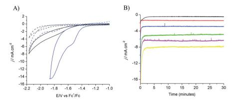
Fig. 1 (A) Cyclic voltammograms recorded on a modified Cu electrode (80 s electrodeposition) (blue) and Cu plate electrode (black) in  $[EMIM](BF_4)/H_2O$  (92/8 v/v) after  $N_2$  purging (dashed lines) and  $CO_2$  purging (solid lines). (B) Current densities during electrolysis in  $CO_2$ -saturated  $[EMIM](BF_4)/H_2O$  (92/8 v/v) at different potentials: -1.25 V (black), -1.35 V (red), -1.45 V (blue), -1.55 V (green), -1.65 V (magenta), and -1.75 V (yellow) vs.  $Fc^+/Fc$ .
