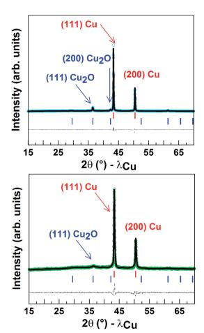
Fig. 5 Rietveld refinement of X-ray patterns of a powder of the Cu porous material (80 s electrodeposition) before (top) and after (below)  $\mathrm{CO}_2$  electroreduction. The observed (open circles), calculated (black line) and difference (blue line on top and green line on bottom) patterns are shown. The red and blue vertical tick bars represent the Bragg positions for Cu and  $\mathrm{Cu}_2\mathrm{O}$ , respectively.
