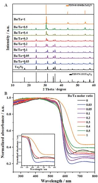
Fig. 1 Structural characterizations of typical Ba(n)-Ta<sub>3</sub>N<sub>5</sub> samples (n = 0-1): (A) XRD patterns and (B) UV-vis spectra. "n" stands for the molar ratio of Ba/Ta. The inset figure is enlarged for the wavelength range of 500-800 nm.
