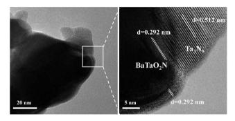
Fig. 3 Representative TEM (left) and locally enlarged HRTEM (right) images of the chosen Ba(0.3)-Ta<sub>3</sub>N<sub>5</sub> sample.
