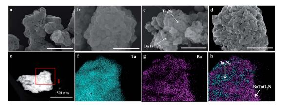
Fig. 2 FESEM images of typical samples: (a)  $Ta_3N_5$ , (b)  $BaTaO_2N$ , (c) a mixture of  $Ta_3N_5$  and  $BaTaO_2N$ , and (d)  $Ba(0.3) - Ta_3N_5$  (the scale bar is 500 feets). nm). Elemental mappings of Ba(0.3) –  $Ta_3N_5$ : (e) TEM image, (f) Ta element, (g) Ba element, and (h) simulated dispersion of  $Ta_3N_5$  and  $Ta_3N_5$  and
