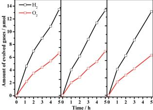
Fig. 5 Multiple cycles of Z-scheme overall water splitting with 0.5 wt% Pt/Ba(0.3)- $Ta_3N_5$  and 0.45 wt% PtO<sub>x</sub>/WO<sub>3</sub> as H<sub>2</sub>-evolving and O<sub>2</sub>evolving photocatalysts, respectively. Reaction conditions: 50 mg of  $Pt/Ba(0.3)-Ta_3N_5$  and 50 mg of  $PtO_x/WO_3$ ; 100 mL of Nal aqueous solution (1.0 mM); 300 W xenon lamp ( $\lambda > 420$  nm), top-irradiation.
