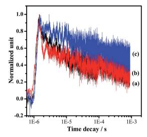
Fig. 6 Normalized transient absorption profiles of the representative samples in a vacuum: (a) Pt/Ta<sub>3</sub>N<sub>5</sub>, (b) Pt/BaTaO<sub>2</sub>N and (c) Pt/Ba(0.3)- $Ta_3N_5$ . The pulse laser at 355 nm was used to excite the samples for the IR tests. The cocatalyst of Pt with a loading amount of 0.5 wt% was deposited by impregnation and a subsequent H<sub>2</sub> reduction method.
