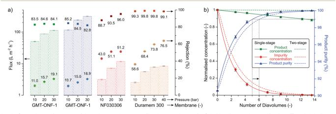
Fig. 6 Separation performance of the solvent-resistant nanofiltration membranes for 2-imidazoline product purification: ■ and ◆ indicates rejections for 1, and the corresponding benzaldehyde substrate impurity, respectively (a). Purification performance for single-stage and two-stage diafiltration processes. Solid and dashed lines represent the simulated performance based on rejections, while symbols signify experimental points to validate the model used for simulation (b).
