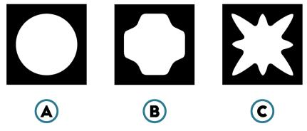
Fig. 4 Void shapes in 2D soft materials. (A) Exhibiting the highest stiffness. (B) Exhibiting the biggest auxetic response. (C) Showing the least compaction with positive Poisson's ratio.<sup>70</sup>
