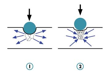
Fig. 2 Deformation profile of (1) non-auxetic material and (2) auxetic material.<sup>25</sup>
