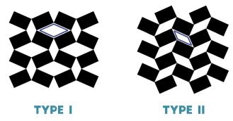
Fig. 10 Type I and Type II rotating rectangles. Type I showing rhombi in their empty space and Type II showing parallelograms.<sup>114</sup>
