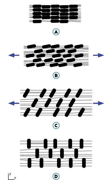
Fig. 6 Structural changes observed in microporous PTFE undergoing tensile loading in the x-direction. (A) Nearly fully densified state. (B) Tension in fibrils causes particle displacement. (C) Rotation of the disc-shaped particles. (D) Fully expanded condition. (B)
