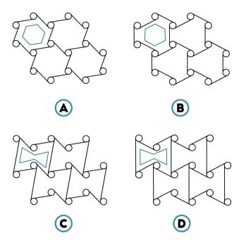
Fig. 8 Chiral structures based on hexagonal and re-entrant hexagonal honeycombs. <sup>102</sup> (A) Trichiral honeycomb. (B) Re-entrant trichiral honeycomb. (C) Anti-trichiral honeycomb. (D) Re-entrant anti-trichiral honeycombs.
