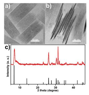
Fig. 1 (a, b) TEM images and (c) XRD pattern of the as-synthesized CeO (CH $_3$ COO) ML nanoplates, the reference pattern in (c) is produced from ref. 41 and 52.
