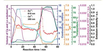
Fig. 3 Time dependence of the emission intensity of Ce<sup>3+</sup> (light blue curve) and Eu3+ (red curve) doped calcium phosphate, in situ ion conductivity (dark blue curve), in situ pH (orange curve) and IR intensity at 1077 cm<sup>-1</sup> (pink curve) in comparison with the volume of the Ca<sup>2+</sup> and Ln<sup>3+</sup> solution (violett curve) to the reactor containing aqueous (NH<sub>4</sub>)<sub>2</sub>HPO<sub>4</sub> (experiments 2 and 6, Table 1).
