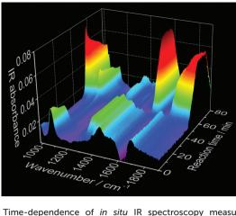
Fig. 4 Time-dependence of in situ IR spectroscopy measurements during the synthesis of Ce<sup>3+</sup>-doped calcium phosphate (experiment 2, Table 1).
