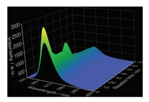
Fig. 6 Time-dependent light transmission of a 365 nm light source during the synthesis of Ce<sup>3+</sup>-doped calcium phosphate (experiment 10, Table 1)
