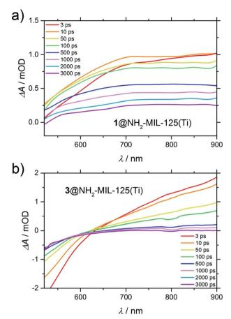
Fig. 7 Difference transient spectra of: (a)  $1@NH_2-MIL-125(Ti)$  in acetonitrile and (b) 3@NH2-MIL-125(Ti) in water upon excitation at 400 nm.
