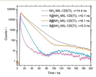
Fig. 5 Time resolved fluorescence of NH<sub>2</sub>-MIL-125(Ti) in water (grey), 1@NH<sub>2</sub>-MIL-125(Ti) in acetonitrile (pink), 2@NH2-MIL-125(Ti) in DMF (orange) and 3@NH2-MIL-125(Ti) in water (blue). The suspensions were excited by a 404 nm laser. The decrease in fluorescence over time was measured at a wavelength of 430 nm and fitted by a sum of exponential decays (only the fastest  $\tau$  component, which is the biggest contribution, is shown for clarity).
