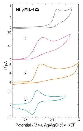
Fig. 4 Cyclic voltammetry at 50 mV s<sup>-1</sup> of NH<sub>2</sub>-MIL-125(Ti), **1**, **2** (phosphate buffer, pH 7) and 3 (0.1 M LiClO<sub>4</sub>) in water as it is the only medium that allowed for electrochemical measurements of the MOF.
