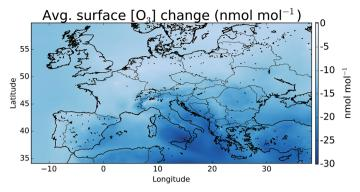
Fig. 7 Difference in surface mean  $O_3$  mixing ratio between "HAL" and "NOHAL" in nmol  $\mathrm{mol}^{-1}$  over the simulation period. Changes in percentage terms are shown in Fig. 8.
