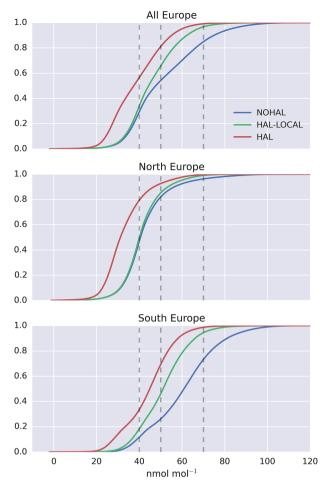
Fig. 9 Cumulative probability distribution plot of surface modelled O<sub>3</sub> for the observation period, for the entire domain (top), northern Europe (>47°N, middle), and southern Europe (<47°N, bottom). Modelled values are shown for the simulation with halogens ("HAL"), without halogens ("NOHAL"), and with halogens only with the European domain ("HAL-LOCAL"). Vertical dashed black lines give 40, 50 and 70 nmol mol<sup>-1</sup>. The x axis is limited to  $120 \text{ nmol mol}^{-1}$
