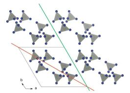
Fig. 1 Schematic of identifying growth planes in ZIF-8. The organic linkers are suppressed and lighting is turned out in VESTA<sup>28</sup> for clarity. Orange: the (110) plane is not allowed, as it cannot be drawn without dissecting linker units. Green: the (100) plane is allowed as it can be drawn without dissecting linker unit.
