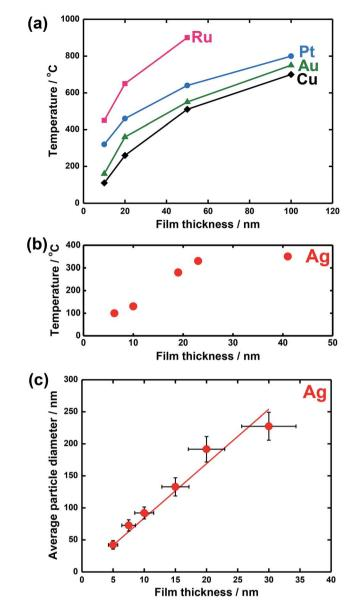
Fig. 4 Some examples of parameter effects:  $T_{\rm dewet}$  for (a) island formation in Ru, Pt, Au, and Cu films and (b) in a Ag film as a function of film thickness; (c) average particle size for fully dewetted Ag films as a function of film thickness. Fig. (a) is reprinted with permission from ref. 61. Copyright 2005, American Vacuum Society; Fig. (b) is reproduced from ref. 62 with permission of Springer; Fig. (c) is reproduced from ref. 63 with permission of IOP Publishing.
