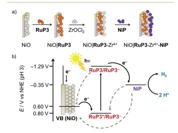
Fig. 2 (a) Supramolecular dye–catalyst assembly on photocathode: layer-by-layer deposition of RuP3,  $\rm Zr^{4+}$  and NiP on p-type NiO photocathode (see text for details). (b) Energy diagram of the NiO photocathode assembly showing the proposed electron transfer mechanisms (reductive quenching) as black solid arrows and possible recombination pathways as grey dashed arrows between p-NiO, RuP3 and NiP.
