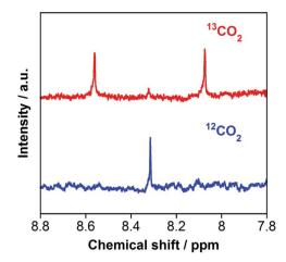
Fig. 3  $^{1}$ H NMR spectra of the aqueous reaction solutions (1 mL) containing RuRu/Ag/TaON (4 mg) and EDTA·2Na (10 mM), measured after 24 h irradiation at  $\lambda_{\rm ex}$  > 400 nm under  $^{13}$ CO<sub>2</sub> (red) and  $^{12}$ CO<sub>2</sub> (blue) atmospheres.
