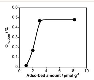
Fig. 5 Relationship between  $\Phi_{\mathsf{HCOOH}}$  and loading amount of RuRu in the photocatalytic reaction using RuRu/Ag/TaON (30 mg) and EDTA·2Na (10 mM) in aqueous solution (10 mL) with 400 nm monochromatic light irradiation under a CO2 atmosphere.
