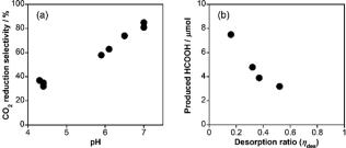
Fig. 4 (a) Selectivity of  $CO_2$  reduction ( $sel_{CO_2}$ ) vs. pH of the reaction solution in the photocatalytic reactions. (b) Produced amount of HCOOH  $\emph{vs.}$  desorption ratio of RuRu ( $\eta_{des}$ ) by the photocatalytic reactions with various concentration of NaH<sub>2</sub>PO<sub>4</sub> (pH = 4.4).
