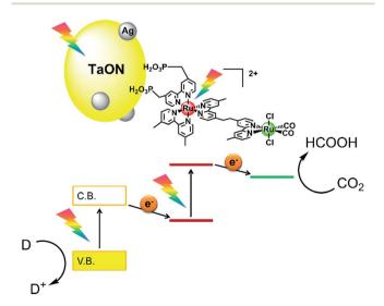
Scheme 1 Hybrid powder photocatalyst of the Ru(II) binuclear complex adsorbed on Ag-modified TaON (RuRu/Ag/TaON).
