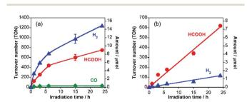
Fig. 2 Time courses of HCOOH (red), H $_2$  (blue) and CO (green) formation by visible-light ( $\lambda$  > 400 nm) irradiation to RuRu/Ag/TaON (4 mg) in EDTA·2Na (10 mM) aqueous solution (4 mL) without (a) and with (b) Na $_2$ CO $_3$  (0.1 M) under a CO $_2$  atmosphere.
