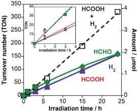
Fig. 6 Time courses of HCOOH (red), H<sub>2</sub> (blue) and HCHO (green) formation along with the sum of HCOOH and H2 (black broken line) in the photocatalytic reaction: RuRu/Ag/TaON (4 mg) in a H<sub>2</sub>O-MeOH (4:1 v/v) mixed solution (4 mL) was irradiated by visible light  $(\lambda > 400)$ nm) under a CO<sub>2</sub> atmosphere. Inset shows enlarged time courses until 4 h irradiation.
