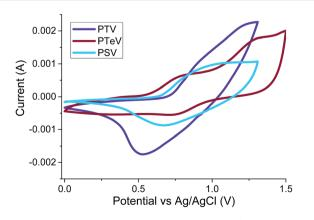
Fig. 3 Thin-film cyclic voltammograms of P3TV, P3SV and P3TeV on Pt electrodes in  $CH_3CN/0.1 \text{ M} [nBu_4N]^+[PF_6]^-$  at 50 mV s<sup>-1</sup>.
