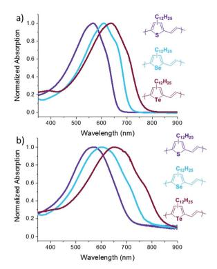
Fig. 2 UV-Vis spectra of P3TV. P3SV and P3TeV in dilute chlorobenzene (a) and in thin films (b)
