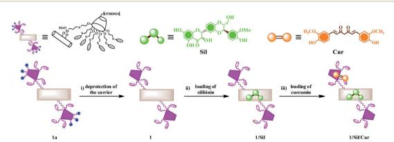
Fig. 2 Schematic representation of synthetic route to halloysite nanotube-cyclodextrin hybrids loaded with silibinin and curcumin.
