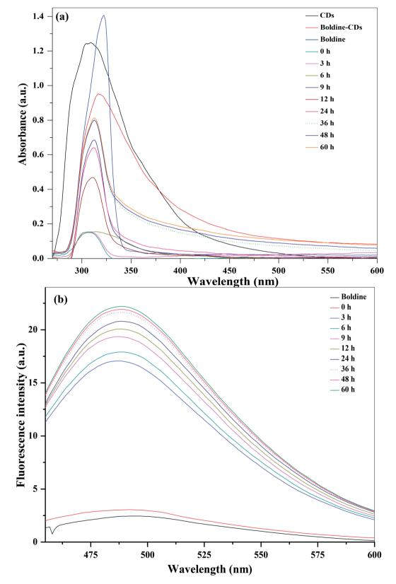
Fig. 3 (a) UV-visible and (b) emission spectra of boldine-loaded CDs at different time intervals from 0 to 60 h in PBS buffer at pH 5.2. Boldine responses for  $327.27 \, \mu g \, mL^{-1}$  boldine-loaded CDs under 430 nm excitation.
