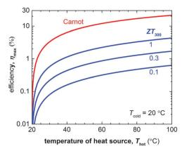
Fig. 15 The Carnot efficiency (red) and maximum efficiency  $\eta_{\text{max}}$  of a thermoelectric leg (blue) with increasing heat source temperature  $T_{hot}$ (the heat sink is kept at  $T_{\rm cold}$  = 20 °C). Eqn (8) was used to calculate  $\eta_{\rm max}$  for materials with a figure of merit at 300 K of  $ZT_{300}$  = 0.1, 0.5 and 1.
