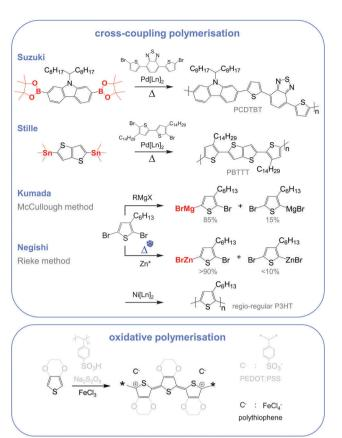
**Fig. 5** Most common reaction schemes for conjugated polymer synthesis include cross-coupling polymerisations (top), where a bifunctionalised monomer (red, boronic ester for Suzuki, organostannyl for Stille, *Grignard* for Kumada and organozinc for Negishi) is polymerised with an aryl halide (mostly an aryl bromide) by the action of a metal catalyst, and oxidative polymerisation (bottom) of 3,4-ethylenedioxythiophene (grey) and thiophene (black) yielding PEDOT:PSS and doped polythiophene.
