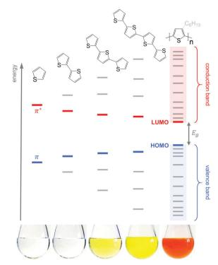
**Fig. 3** Evolution of the HOMO and LUMO levels as well as bandgap  $E_{\rm g}$  with increasing number of thiophene repeat units, resulting in valence and conduction bands for polythiophene; the images of 5 g L<sup>-1</sup> solutions in chloroform illustrate the narrowing of  $E_{\rm g}$ , which leads to a red-shift in absorption (the polymer is P3HT). Note that crystallisation will lead to a further decrease in  $E_{\rm g}$  due to electron delocalisation across adjacent chain segments.
