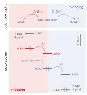
Fig. 9 Basic principle of acid-base doping, which involves the transfer of an anion (A<sup>-</sup>, e.g., H<sup>-</sup>) or cation (C<sup>+</sup>, e.g., H<sup>+</sup>) to the semiconductor (top); and redox doping, which involves the transfer of an electron to the LUMO or from the HOMO of the semiconductor in the case of n- and p-doping. respectively (bottom)
