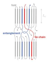
Fig. 7 Schematic nanostructure of a semi-crystalline polymer, indicating a chain fold that re-enters the same crystallite (with lamellar thickness  $L_c$ ), a tie chain that bridges two adjacent crystallites, and a chain entanglement that is trapped in the amorphous region between two crystallites.
