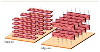
Fig. 8 Face-on (left) and edge-on (right) orientation of a P3HT crystallite with the  $\pi$ -stacking direction lying out-of-plane and in-plane, respectively
